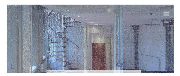
The Autoupdate tool was removed and the previous Density and Realtime Density sliders were replaced by a single Level of Detail slider. The Level of Detail sets the density for all point clouds in the drawing and is relative to the maximum points as specified on the 3D Modeling tab of the Options dialog box. The maximum points displayed on-screen has increased in AutoCAD 2015 from 10 million to 25 million.
