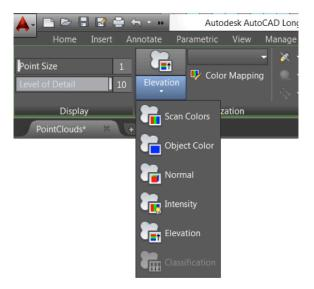
The former Point Cloud Intensity Color Mapping dialog box is replaced with the new Point cloud Color Map dialog box. In it you can select the appropriate tab to customize the colorization based on intensity, elevation, or classification. You can select from predefined color schemes or create and save your own.
