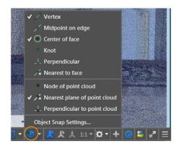
You can snap to points on the point cloud with the Node point cloud object snap. If the point cloud has segmentation data, you can snap to the nearest point on planar segments or perpendicular to planar segments.
