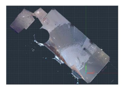
After specifying an appropriate cropping boundary from one view (such as plan), change to another view (such as elevation) to intuitively specify the cropping boundary for the height. You can continue to change views and create cropping boundaries to focus on just the area of the point cloud that you need.
