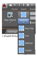
Slider bars on the Map Image Ribbon tab enable you to adjust the brightness, contrast, and fading of the map image so that you can more easily see relevant AutoCAD geometry.
