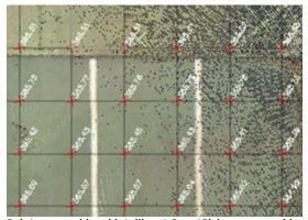
Points on a grid and intelligent SmartPick snaps provide a highly productive automated surveying tool used to create COGO points most typically used for generate a ground surface TIN.
