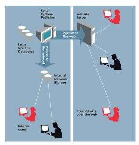
Leica Cyclone Publisher is used to compress point cloud data and create panoramic images with accurate measurable data for viewing and markup with the free TruView Internet Explorer plug-in. This data, much like PDF, can be made available on an internal network, over the web or distributed on a CD or DVD. The TruView plug-in makes accessing this data easy for any class of user, with no training required.
