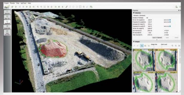
**The rayCloud editor** combines the 3D point cloud with the original images and is a ground-breaking concept that offers you a completely new viewing and annotating experience. Use the rayCloud editor to view, assess, interpret and improve the quality and accuracy of your results. And measure, vectorize, classify and perform GIS and CAD functionalities directly in the rayCloud editor.
