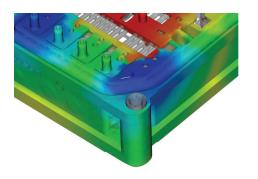
Two-shot sequential overmolding Simulate the two-shot sequential overmolding process: one part is filled; the tool opens and indexes to a new position; and a second part is molded over the first.
